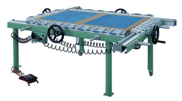
The HYBRID SCREEN is a mesh stretcher hybrid (manual system / pneumatic) equipped with 4 tension bars assemble in a feet structure. The HYBRID SCREEN is ideal for a intensive using and is capable to stretch several screen with different formats in one single time. The HYBRID SCREEN as the possibility to adjust to several sizes by moving 2 bars in a single adjusting movement. The 2 stretching bars that moves are equipped with wheels for better and easy moving.
