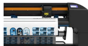
ORANGE status = Lift pinch rollers
