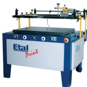
Manual printing machines with guide arm and paralell opening available
