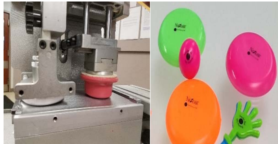
Figure 2: Silicone pad and finished pieces
