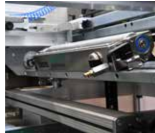
Screen clean • Automatic screen humidification (screen clean) • Removes dried paint without manual cleaning
