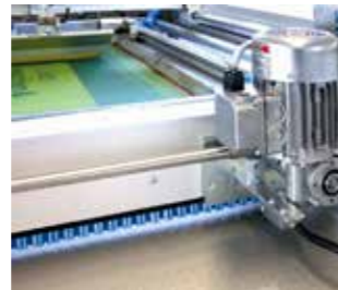
Integrated substrate cleaning • Automatic foil cleaning before printing
