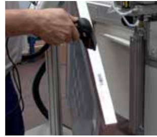
Barcode Handscanner • For documentation of material batches (film, paint) • To call the print program
