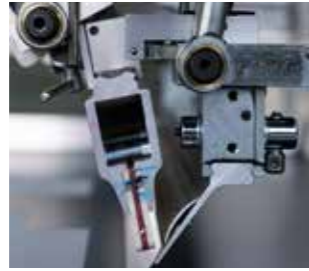
Anti-Drip • Anti-drip for printing and/or flood squeegees
