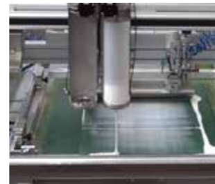
Paste dosing • Pastes are supplied cyclically
