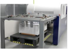
XL PALLET STACKER Based on offset models, it simplifies pallet unloading and production workflows. Supports sheets up to size 75x120 cm (29x47")
