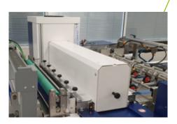
NEW CTS XL MODULE (electrode ceramic technology) In-line system made to optimize the varnish quality on special substrates
