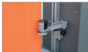
Encoder to accurately measure the rewound length of the material
